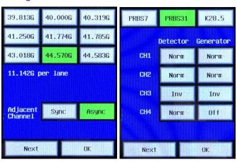
The four channels can be configured to operate synchronously to each other or the odd/even channels configured to operate asynchronously. In asynchronous operation
