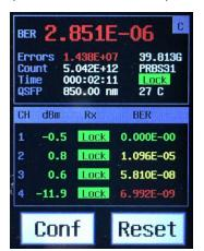
Upon exiting the configuration screen, the Eye-BERT 40G begins monitoring and displaying the bit error rate and QSFP measurements. Status and BER measurements for each of the four channels are displayed separately
